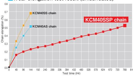
\* SS, AS, and SSP were all tested under the same condition. Condition: load at 440N (maximum allowable tension for 40SS)
