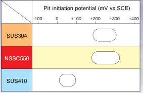
Excerpt from a material for NSSC550 supplied by Nippon Steel Stainless Steel Corporation
